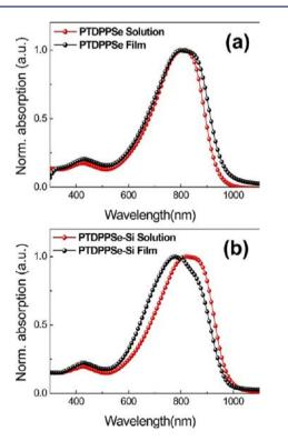
**Figure 2.** UV–vis–NIR absorption spectra of (a) **PTDPPSe** and (b) **PTDPPSe-Si** in dilute chlorobenzene solution and thin films on a quartz plate.
