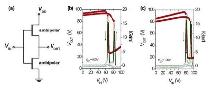
Figure 7. (a) Schematic of the complementary inverter structure. CMOS-like inverter characteristics of (b) PTDPPSe and (c) PTDPPSe-Si inverter ( $V_{DD} = 100 \text{ V}$ ).
