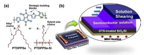
Figure 1. Design motif and solution-shearing schematic. (a) Molecular structures of PTDPPSe and PTDPPSe-Si and (b) schematic illustration of TFT structure and solution-shearing technique, in which a small volume of organic or polymer semiconductor solution is sandwiched between two preheated silicon wafers that move relative to each other at a controlled speed. This method yields crystalline and aligned thin films from various soluble organic or polymer semiconductors.
