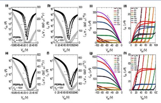
**Figure 6.** Current–voltage (I-V) characteristics of TFTs. {(a)–(d)} **PTDPPSe** and {(e)–(h)} **PTDPPSe-Si** solution-sheared thin films annealed at 220 °C. Transfer characteristics at {(a),(e)} hole-enhancement operation,  $V_{DS} = -100$  V, and {(b),(f)} electron-enhancement operation,  $V_{DS} = 100$  V. {(c),(d),(g), and (h)} Output characteristics of TDPP-selenophene copolymers ( $L = 50 \mu m$  and  $W = 1000 \mu m$ ).
