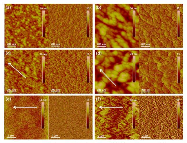
Figure 5. AFM height (left) and phase (right) images of  $\{(a),(c),(e)\}$  PTDPPSe and  $\{(b),(d),(f)\}$  PTDPPSe-Si films by  $\{(a),(b)\}$  drop-casting and  $\{(c)-(f)\}$  solution-shearing methods after annealing at 220 °C. The arrow indicates the direction of shearing.
