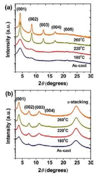
Figure 4. Out-of-plane X-ray diffraction (XRD) patterns of (a) PTDPPSe and (b) PTDPPSe-Si thin films, depending on annealing temperature.
